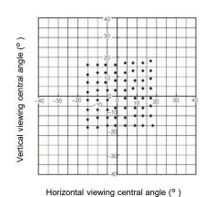
(2) Each pixel's viewing angle (half angle)
