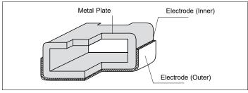
The electrodes (internal and external electrodes) of EYF3CU are entirely formed on the outer surface by plating. The inner wall and the end surfaces are not plated.
