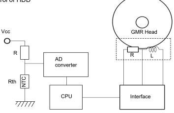
Temperature compensation (Pseudo-linearization) Contrast level control of LCD
