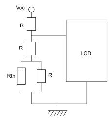
Temperature compensation (RF circuit)
