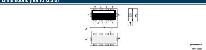
Mass **Dimensions** Part No. (Weight) (inch size) (g/1000 pcs) L W b d Τ а е **EZAEGCA50AV**  $2.0 \pm 0.1$  $1.25 \pm 0.10$ (0.5) $0.30 \pm 0.15$  $0.25 \pm 0.15$  $0.20 \pm 0.15$  $0.35 \pm 0.15$  $0.50 \pm 0.10$ 4.0 (0805)
