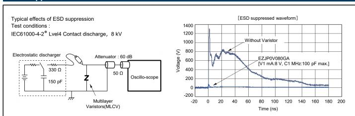
International Standard of the ESD testing method (HBM) for electronic equipment ability to \*IEC61000-4-2 ... withstand ESD generated from a human body. It sets 4 levels of severity
