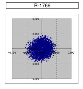
positioning accuracy: 53.7 micron
