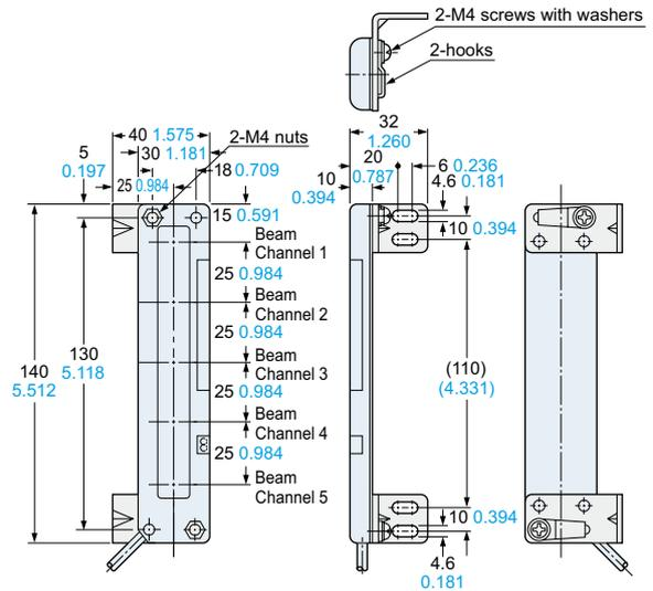
Material: Cold rolled carbon steel (SPCC)
