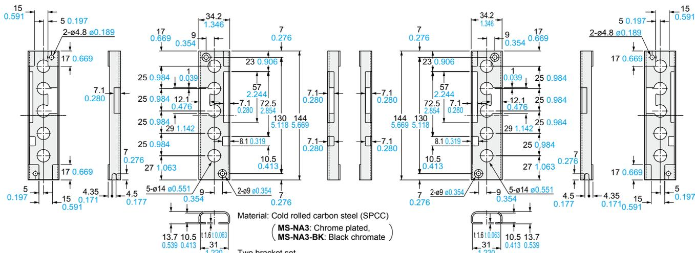
Material: Cold rolled carbon steel (SPCC)
