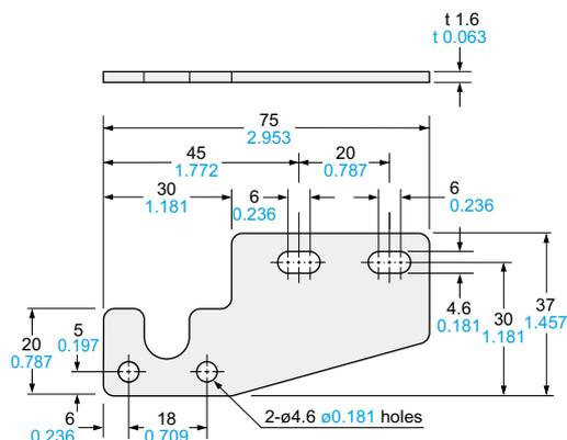
Material: Cold rolled carbon steel (SPCC)
