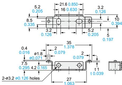
Material: Cold rolled carbon steel (SPCC)
