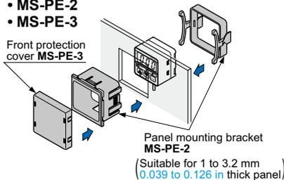
Panel mounting bracket **MS-PE-2**
