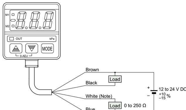
Note: The white lead wire is equipped only with the **DP-M2A**.
