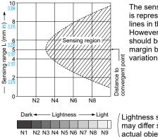
The sensing region (typical) is represented by oblique lines in the left figure. However, the sensitivity should be set with enough margin because of slight variation in products.
