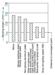
The bars in the graph indicate the sensing range (typical) for the respective material. However, there is a slight variation in the sensing range depending on the product. Further, if there is a reflective object (conveyer, etc.) in the background of the sensing object, since it affects the sensing, separate it by more than twice the sensing range shown in the left graph.
