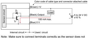
incorporate a reverse polarity protection circuit.
