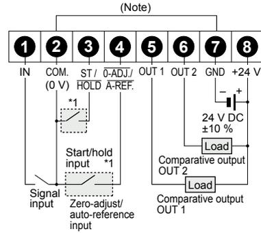
Note: COM. (0 V) is internally connected to GND.
