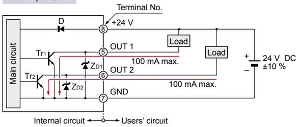
Symbols ... D: Reverse supply polarity protection diode
