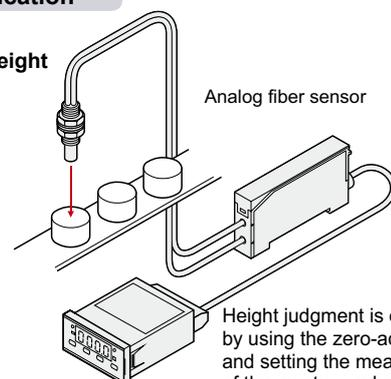
Height judgment is easily done by using the zero-adjust function and setting the measured values of the master workpiece as “0”.
