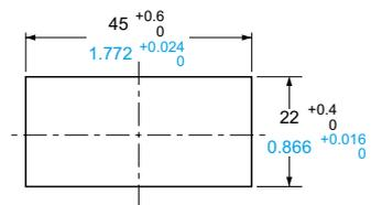
Note: The panel thickness should be 0.5 to 4 mm
