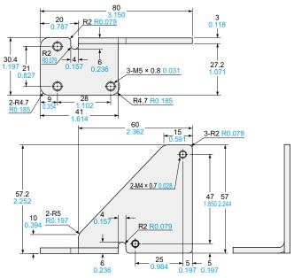
Material: Stainless steel (SUS) Two M4 (length 30 mm 1.181 in) screws with washers are attached.
