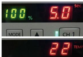
While the display is showing irradiation conditions, you can see the temperature of the LED head simply by pressing the MODE button. The controller is designed to dissipate heat, and it is easy to estimation of life.
