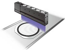
Curing and separation of dicing film and BG film
