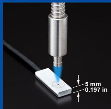
The UV intensity can be relative measured<sup>(Note 1)</sup> at the actual position by using the slim UV sensor. It can also automatically adjust the UV intensity to the preset level. Since the sensor only has 5 mm (0.197 in) thickness, which is similar to the workpiece, the intensity measurement is possible without removing the system from the production line, facilitating
