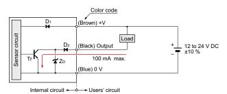
D1: Reverse supply polarity protection diode Symbols .. D2: Reverse output polarity protection diode ZD: Surge absorption zener diode Tr : NPN output transistor
