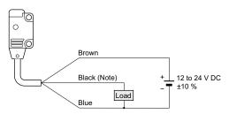
Note: The emitter of the thru-beam type sensor does not incorporate the black wire
