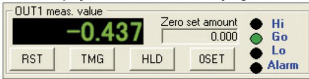
Missing and loose screws can be detected by sensing the displacement of the screw head from the reference plane. **HL-D3** provides Hi / Go / Lo judgment based on the sensing results.
