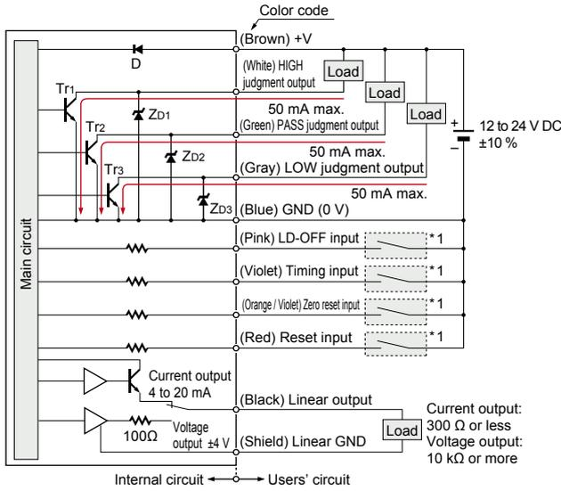
Symbols ... D: Reverse supply polarity protection diode
