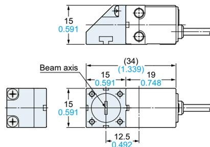
**HL-T1SV2**Side-view attachment for **HL-T1010A(F)** (Optional)**Assembly dimensions**Mounting drawing with **HL-T1010A**'s receiver
