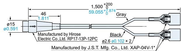
\* The sensor heads that were produced before January 2006 use the connector shown below. Please note that the new connector and previous connector are incompatible.
