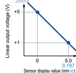
The linear output must be set by determining output values (maximum; current: 0 to 23.5 mA / voltage:  $\pm 5.5$  V) at two different points, for the arbitrary display value.
