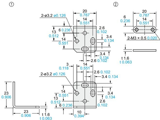
Material: Cold rolled carbon steel (SPCC) (Uni-chrome plated)
