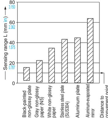
The bars in the graph indicate the sensing range (typical) for the respective material. However, there is a slight variation in the sensing range depending on the product. Further, if there is a reflective object (conveyor, etc.) in the background of the sensing object, since it affects the sensing, separate it by more than twice the sensing range shown in the left graph.
