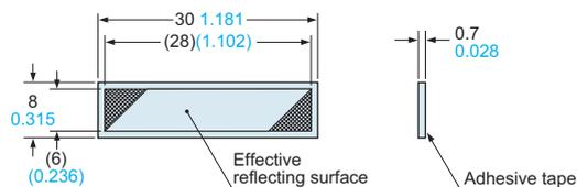
Material: Flexible polyvinyl chloride
