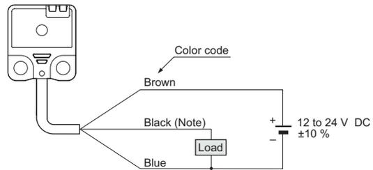
Note: The emitter of the thru-beam type sensor does not incorporate the black wire.
