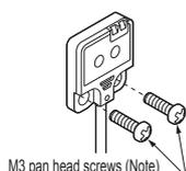
Note: When mounting the front sensing type sensor, use M3 pan head screws without washers, etc.
