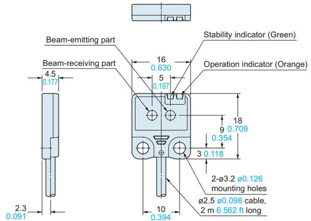
**RF-200** Reflector (Accessory for the retroreflective type sensor)
