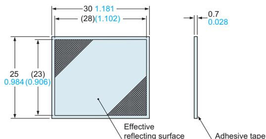
Material: Flexible polyvinyl chloride
