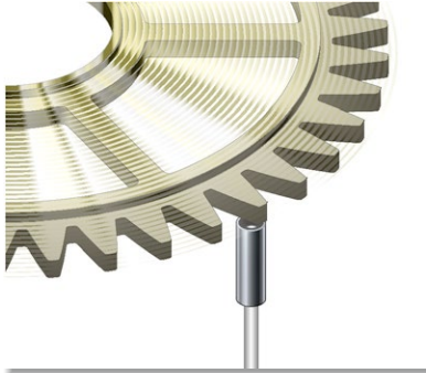
Detecting rotation of a gear
