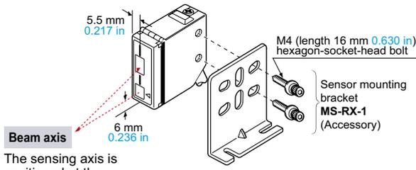
The sensing axis is positioned at the intersection of the "Δ" mark on the lens face and the "I" line.
