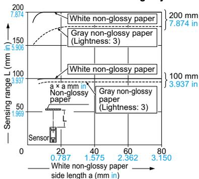
These curves show the characteristics with the maximum sensing range set to 100 mm 3.937 in, 200 mm 7.874 in, each, with white non-glossy paper (50 x 50 mm 1.969 x 1.969 in).
