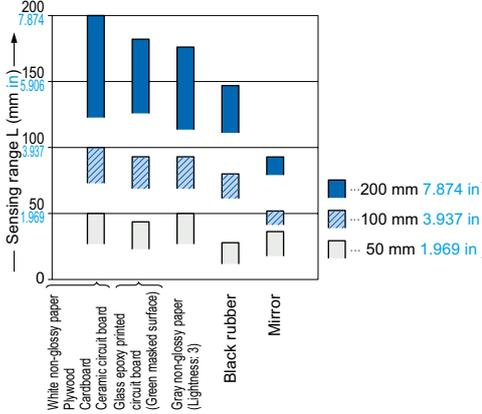
These bars indicate the sensing range with respective objects when the distance adjuster is set at the sensing range of 200 mm 7.874 in, 100 mm 3.937 in and 50 mm 1.969 in long, each, with white non-glossy paper.
