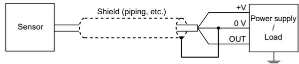
Note: The shield (piping, etc.) must be insulated.
