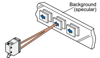
(However, changing the angle of the sensor is necessary when the background object has a specular surface.)
