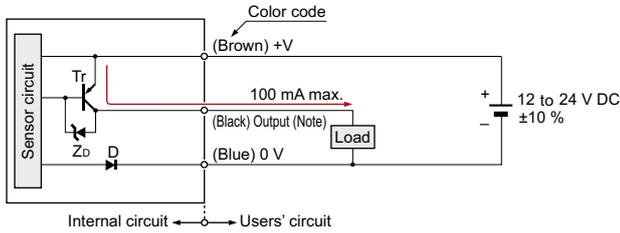
Note: The output does not incorporate a short-circuit protection circuit.
