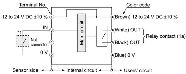
Note: The output does not incorporate a short-circuit protection circuit.
