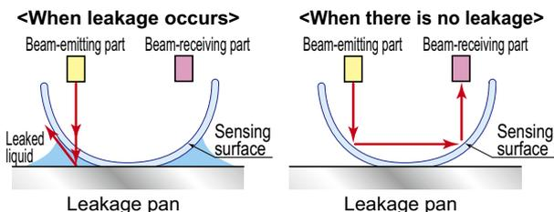
The beam from the beam-emitting part scatters through the leaked liquid and is not transmitted to the beam-receiving part.
