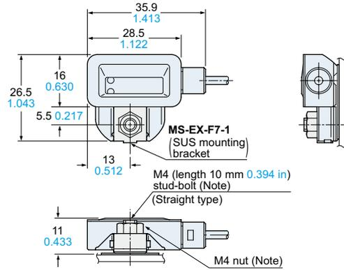
Note: A M4 stud-bolt has been welded to this unit.
