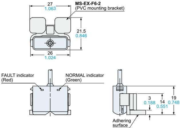
**EX-FC1** Simple wire-saving unit for leak detection sensor
