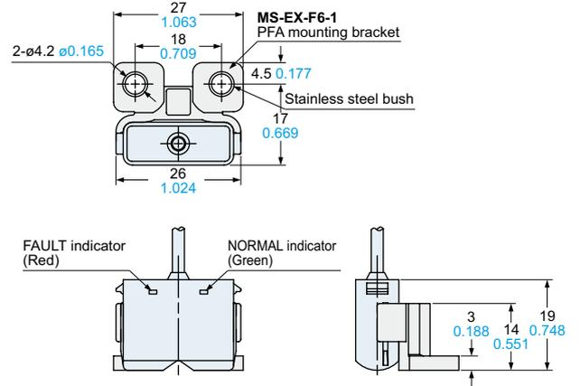
**Assembly dimensions with mounting bracket for EX-F62(-PN)**
