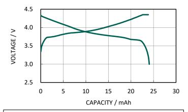
Charge Condition: CC/CV 22.0mA(1C) - 4.35V, 1.1mA(0.05C) cut-off at 20°C Discharge Condition: CC, 4.4mA(0.2C) - 3.0V cut-off at 20°C
