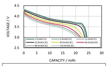
Charge Condition: CC/CV 11.0mA(0.5C) - 4.35V, 1.1mA(0.05C) cut-off at  $20^{\circ}$ C Discharge Condition: CC, 3.0V cut-off at  $20^{\circ}$ C
