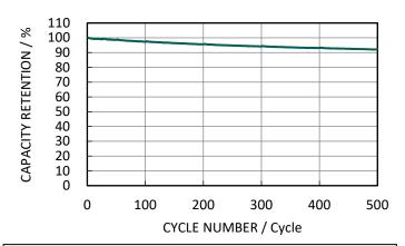
Charge Condition: CC/CV 22.0mA(1C) - 4.35V, 1.1mA(0.05C) cut-off at 20°C Discharge Condition: CC, 22.0mA(1C) - 3.0V cut-off at 20°C
