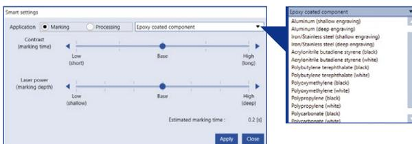
The knowhow of setting marking conditions such as laser power, scan speed and pulse frequency is packed in the software. The software lets the user select desired marking condition from the 15 material types with a one-touch operation.
