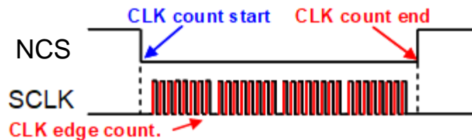
Figure 5-7 SCLK Bit Count Timing
