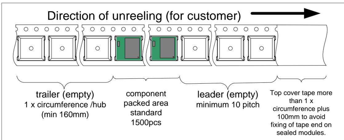
Empty spaces in the component packed area shall be less than two per reel and those spaces shall not be consecutive.
