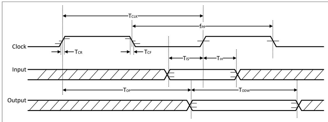
**SDIO Timing Data – DDR50 Mode ( $V_{IO\text{SD}} 1.8\text{ V}$ )**
