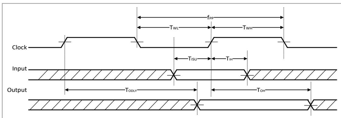
**SDIO Timing Data – SDR12, SDR25, SDR50 Modes (V<sub>IOSD</sub> 1.8 V)**
