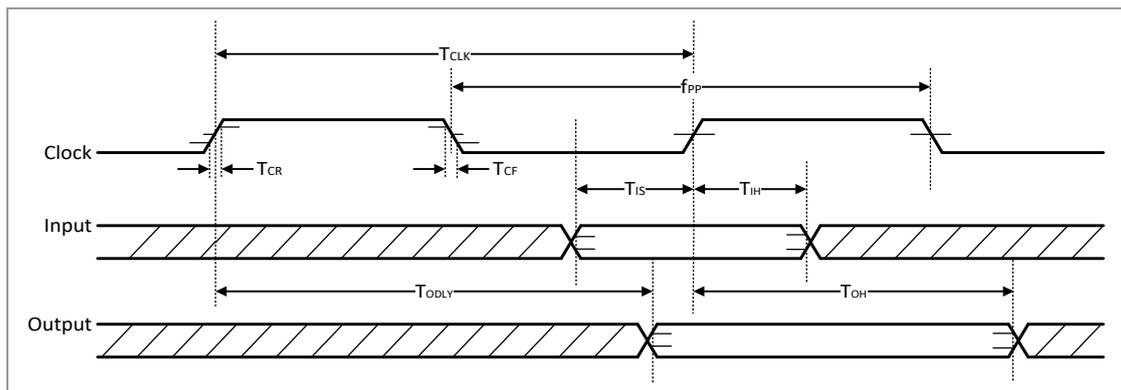
**SDIO Timing Data – SDR104 Mode (V<sub>IOSD</sub> 1.8 V)**
