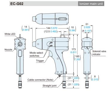
Note: An exclusive intermediate cable (oil-resistant, heat-resistant, bendingresistant type, ø3.7 mm ø0.146 in, 2 m 6.562 ft long) is attached.
