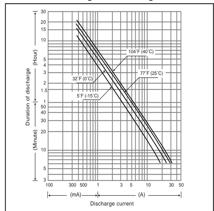
(Note) The above characteristics data are average values obtained within three charge/discharge. Cycles not the minimum values.
