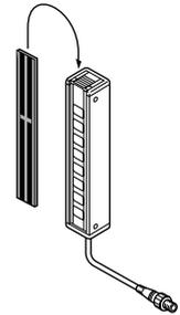
The slit mask restrains the amount of beam emitted or received and hence reduces the interference between neighbouring sensors. Replace the original front cover with the slit mask. However, the sensing range reduces when the slit mask is used.
