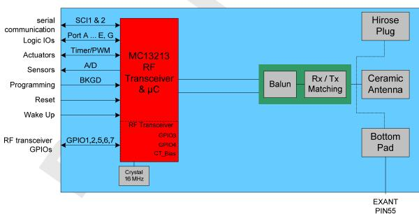
The MC13213 is used in single port configuration with its internal Tx/Rx switch. For more details refer to chapter 7.1.
