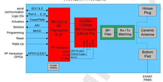
The RF frontend IC CC2591 / CC2590 is controlled with GPIO3, GPIO4 and CT\_Bias from RF transceiver unit (see above block diagram).
