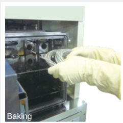
Vacuum baking for the reduction of outgas
