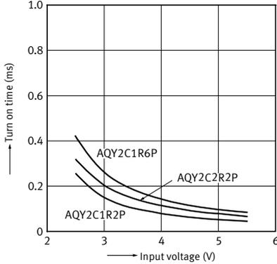
11-2. Turn on time vs. input voltage characteristics
