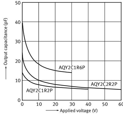
13-2. Output capacitance vs. applied voltage characteristics
