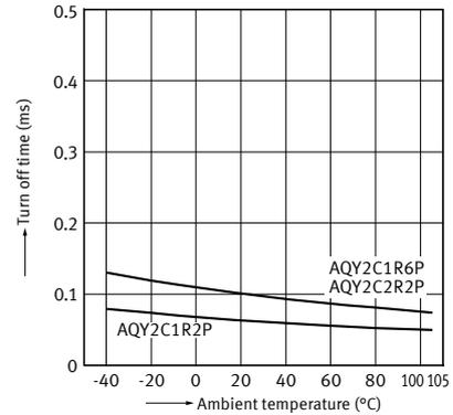
4-2. Turn off time vs. ambient temperature characteristics
