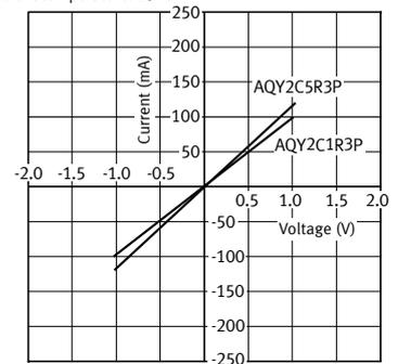
9. Input current vs. input voltage characteristics
