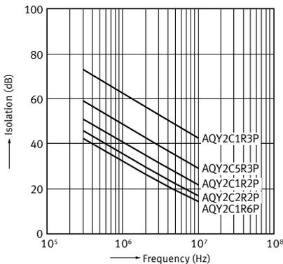
15. Insertion loss vs. frequency characteristics (50Ω impedance)
