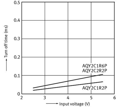
12-2. Turn off time vs. input voltage characteristics
