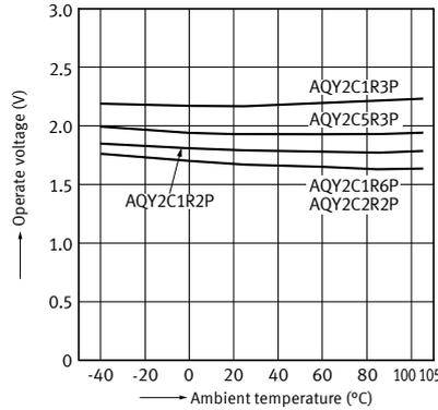
6. Turn off voltage vs. ambient temperature characteristics
