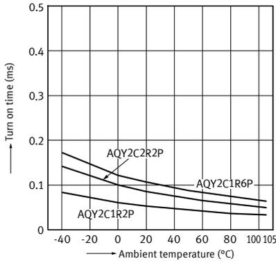
**3-2. Turn on time vs. ambient temperature characteristics**
