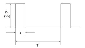
$P_{P}$ : Pulse limit power (W) : Pulse limit voltage (V) : Pulse continuous time (s)
