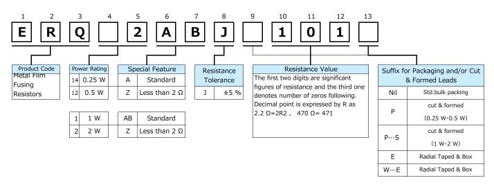
The above example shows a standard Metal Film Fusing Resistors, 2 W power rating, resistance value of 100  $\Omega$ , tolerance of  $\pm 5$  %, and package of standard bulk packing.
