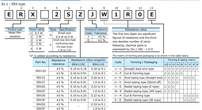
The above example 1 shows a small metal film resistor, 2 W power rating, resistance value of 1.0  $\Omega$ , tolerance  $\pm 5$  %, and package of radial taping.
