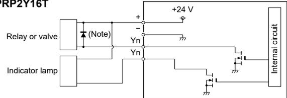
Note: Attach diodes to absorb counter electromotive force from inductive load.
