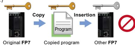
Any attempt to copy the installed equipment's program into a newly purchased FP7 will fail due to an unmatched decryption key, resulting in the equipment becoming inoperable.
