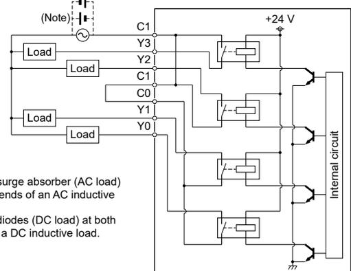
Note: Attach surge absorber (AC load) at both ends of an AC inductive load. Attach diodes (DC load) at both ends of a DC inductive load.
