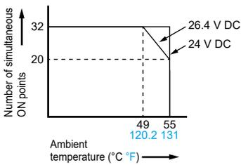
Reduce load current according to the graph below by the external power supply voltage.
