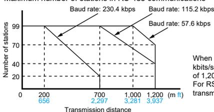
When using a transmission speed of 38.4 kbits/sec. or less, you can set up a maximum of 1,200 m 3,937 ft and 99 units.
