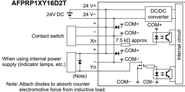
Note: Attach diodes to absorb counter electromotive force from inductive load.
