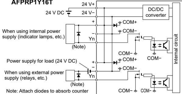
Note: Attach diodes to absorb counter electromotive force from inductive load.
