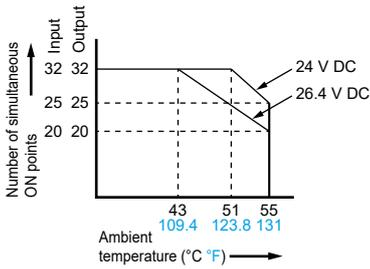
Reduce load current according to the graph below by the external power supply voltage.
