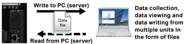
Transfer electric power data from factories and offices to an FTP server on a regular basis.
