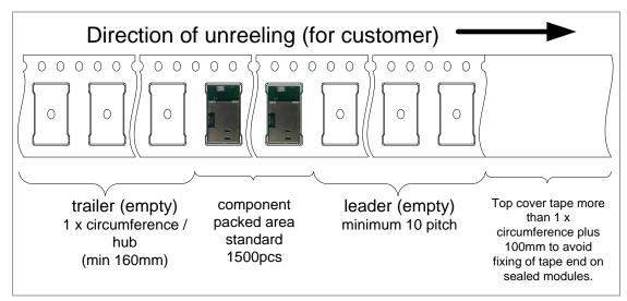
Empty spaces in the component packed area shall be less than two per reel and those spaces shall not be consecutive.
